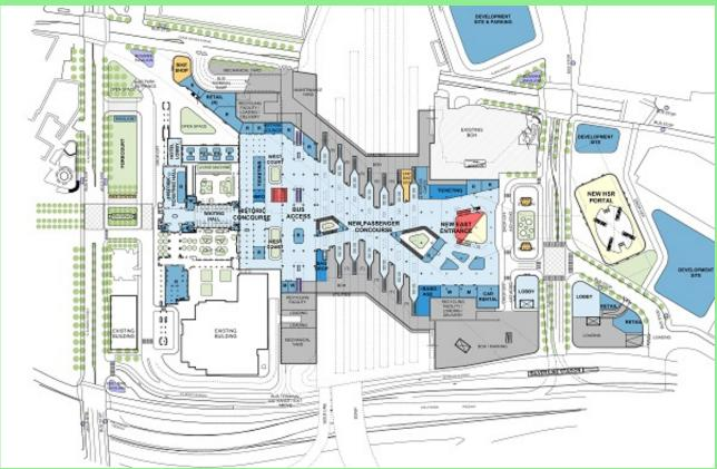
This is the latest plan for the modernization of Los Angeles Union Station. This includes replacing the tunnel to the platforms with an new, large concourse largely sunlight, a new bus station on the northside of the station and creating a landscaped area in the parking lot in front of the station. A new HSR station is planned just east of the current station along with new commercial buildings.
