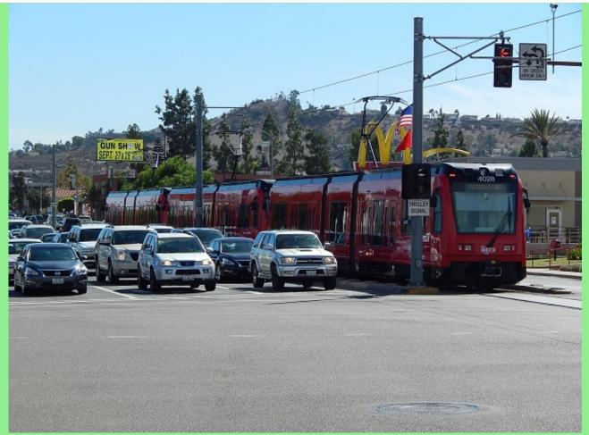
This is in Santee. Here the San Diego Trolley Green Line runs 4 times an hour in each direction on a section of single track in the median of Cuyamaca Street for a distance of almost a half mile. Another example of an economical way to serve areas with Light Rail. Photo by Noel T. Braymer
