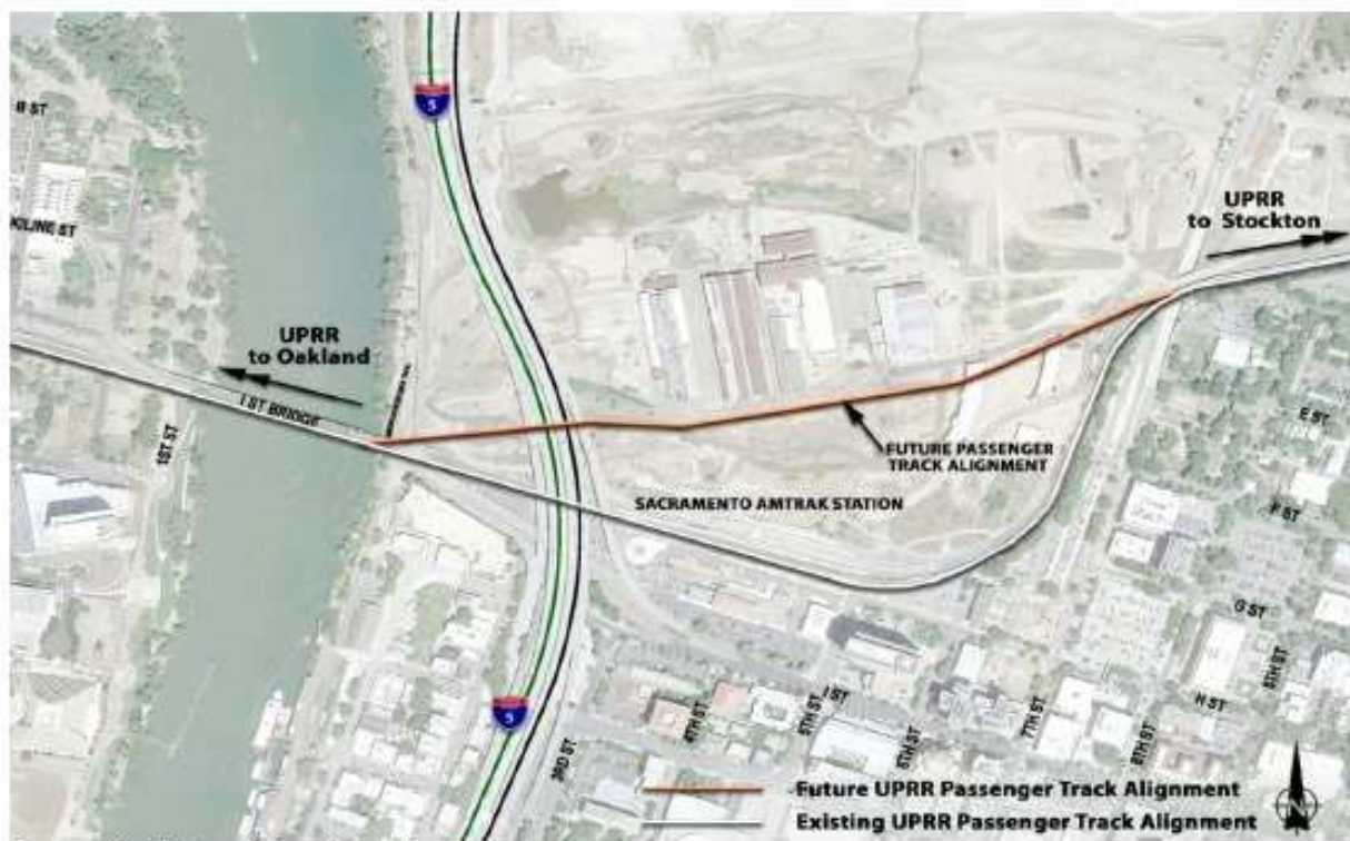
Figure 1-23: Sacramento Amtrak Station – Future Track Relocation
