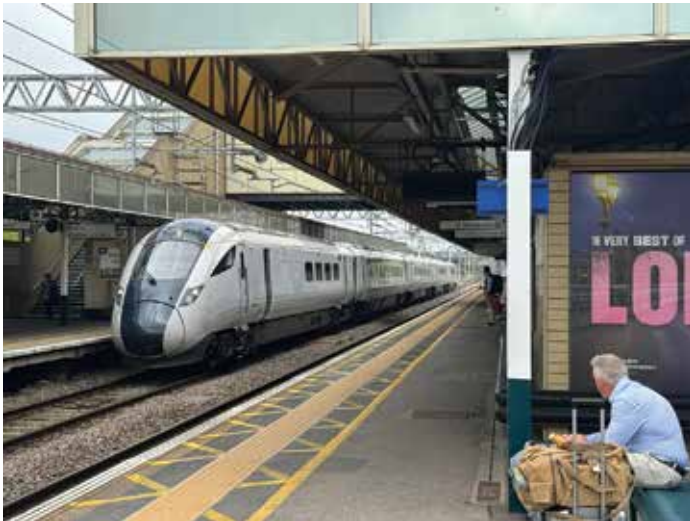
New class 805 Hitachi bi-mode (diesel and electric) 125mph train undergoing mileage trials at Milton Keynes, May 1, 2024. These trains will operate on routes like London - Chester which are 80% electrified. Battery and Hydrogen were considered but deemed not ready for high speed service. Photo: Paul Dyson
