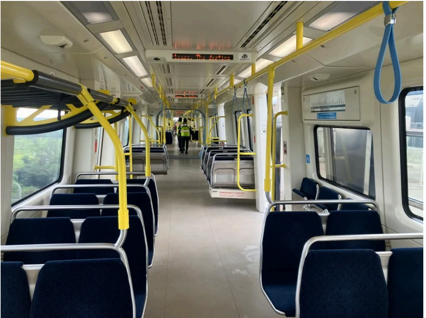
Open gangway interior of Skyline Hitachi Rail Italy train during brief layover at Kualaka'i (East Kapole), the eastern terminus of the line
